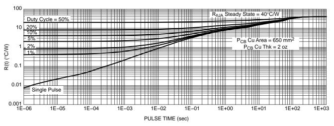
Figure 12. Thermal Impedance (Junction-to-Ambient)
