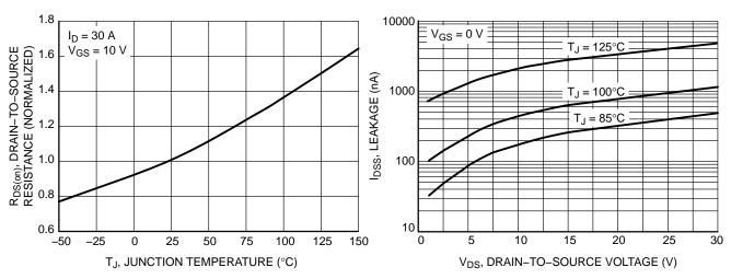
Figure 5. On–Resistance Variation with Temperature
